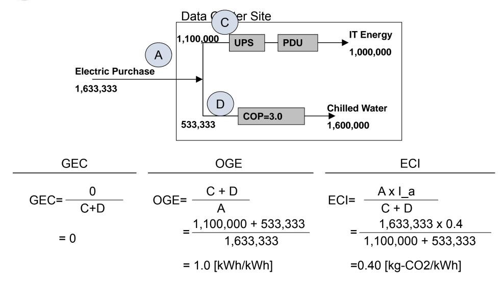
Note: I\_a = 0.4 [kg-CO2/kWh] is the carbon intensity of the grid power in Japan.
