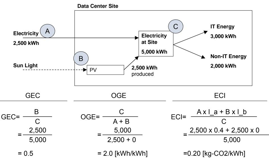
Note: I\_a = 0.4 [kg-CO2/kWh] and I\_b = 0.18 [kg-CO2/kWh] are the carbon intensity of the grid power (A) and natural gas (B), respectively. I\_b = 0.0139 [t-C/GJ] x (44/12) x 0.0036[GJ/kWh] Case E – Electricity & Natural Gas (Cogeneration) Purchase
