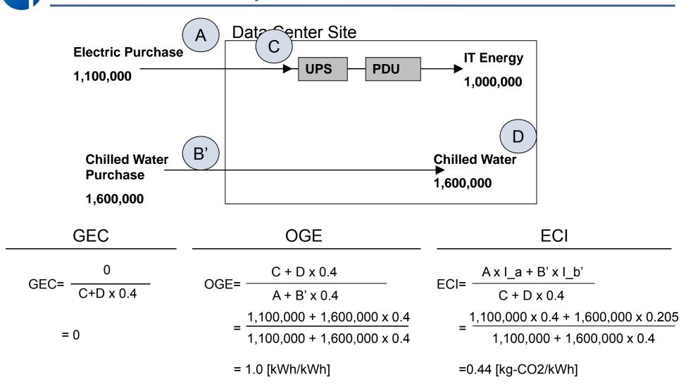
Note: I\_a = 0.4 [kg-CO2/kWh] and I\_b' = 0.205 [kg-CO2/kWh] are the carbon intensity of the grid power (A) and chilled water (B') in Japan, respectively. I\_b' = 0.057 [t-CO2/GJ] x 0.0036[GJ/kWh] Case C – Natural Gas Purchase
