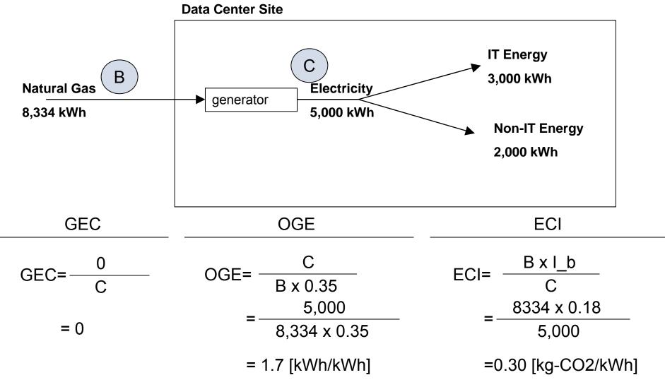
Note:  $I_b = 0.18$  [kg-CO2/kWh] are the carbon intensity of natural gas in Japan. I\_b = 0.0139 [t-C/GJ] x (44/12) x 0.0036[GJ/kWh]
