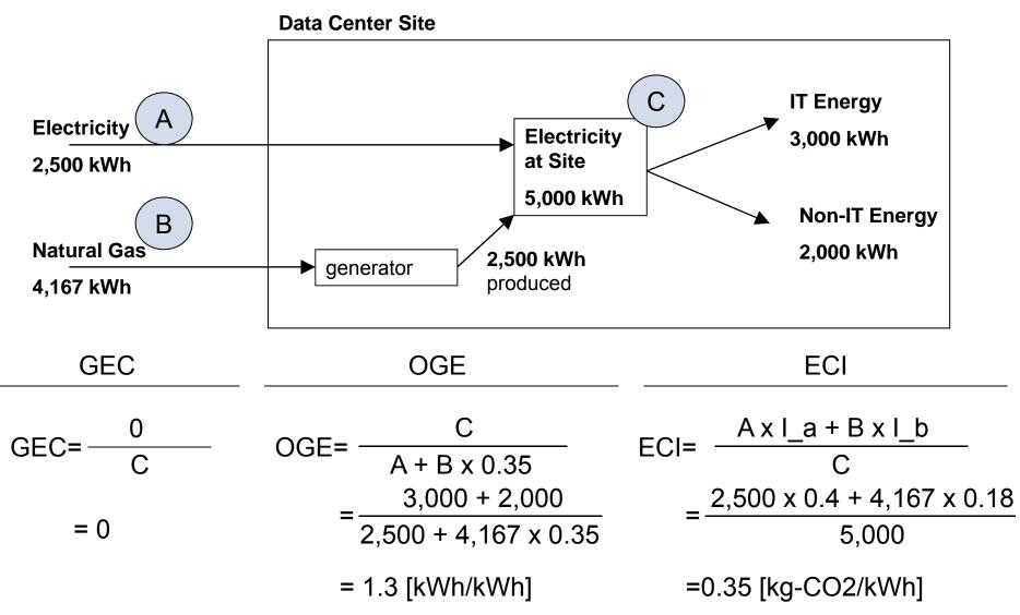
Note:  $I_a = 0.4$  [kg-CO2/kWh] and  $I_b = 0.18$  [kg-CO2/kWh] are the carbon intensity of the grid power (A) and natural gas (B), respectively. I\_b = 0.0139 [t-C/GJ] x (44/12) x 0.0036[GJ/kWh] Case D' – Electric & Photovoltaic (PV)
