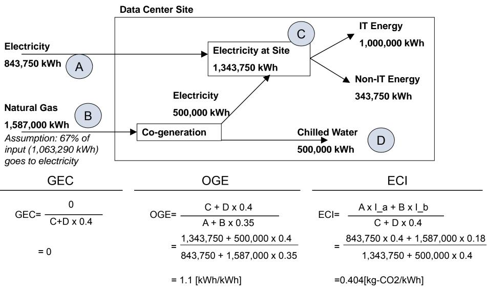
Note:  $I_a = 0.4$  [kg-CO2/kWh] and  $I_b = 0.18$  [kg-CO2/kWh] are the carbon intensity of the grid power (A) and natural gas (B), respectively. I\_b = 0.0139 [t-C/GJ] x (44/12) x 0.0036[GJ/kWh]
