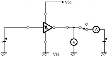
Fig. 1 DC characteristic measurement circuit of Schmitt-trigger input
