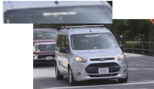
A cyclist is seen from inside the car; the car stops at zebra crossing; the light bar moves outwards and inwards while the cyclist crosses the road, after which bar centralizes, flashes four times, and becomes static when the car starts moving again (Ford Media Center, 2017)
