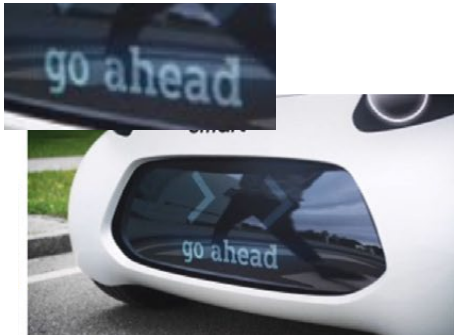
Car moves on road; '11th street' on the bumper, the car stops in front of zebra crossing; 'go ahead' and '>' sign appears on the bumper, and headlights turn into animated eyes; the pedestrian crosses (Daimler, 2017)
