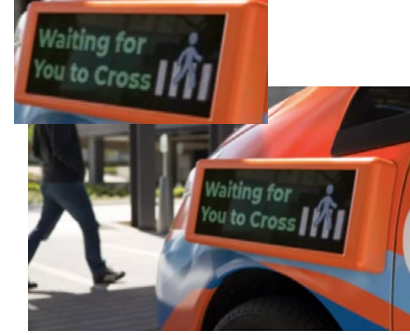
'Waiting for You to Cross' and pedestrian on zebra crossing on car side (drive.ai, 2018)
