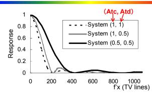
$\checkmark$  The response of System (1, 0.5) is little improved compared with that of System (1, 1), because of the camera response with Atc of 1.
