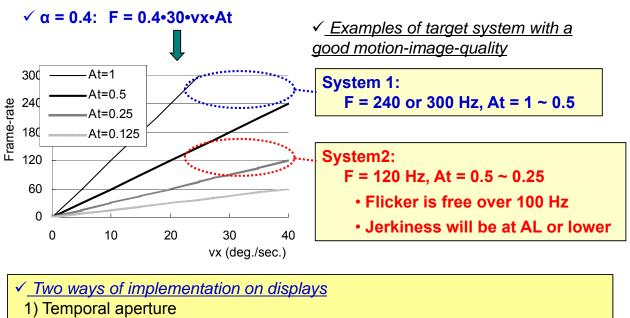
Example: (input) 120 Hz  $\Rightarrow$  (25% scanning BL)  $\Rightarrow$  (display) <u>120 Hz</u>, <u>At=0.25</u> 2) Up-conversion
