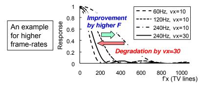
$\checkmark$  Setting frame-rate to extremely high, to overcome the increase of vx, will make devices and systems difficult to realize.
