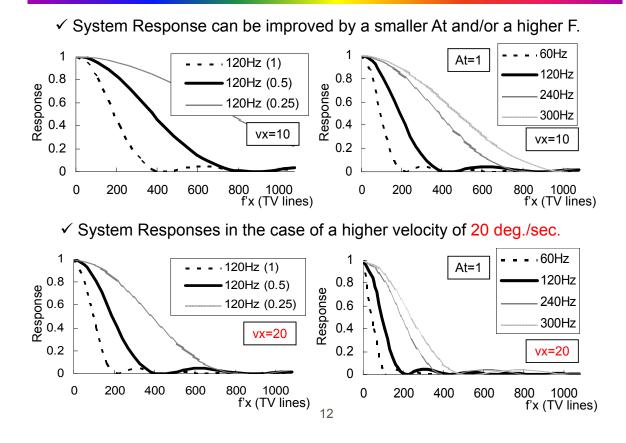
$\checkmark$  A smaller temporal aperture (At) and/or a higher frame-rate (F) can significantly improve system dynamic response.
