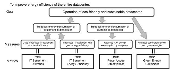
Fig. 2-4: Breakdown of overall datacenter energy efficiency: DPPE
