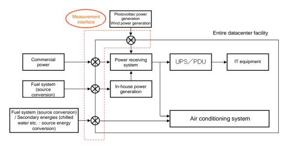
Fig. 2-6: Interface between entire datacenter facility and external area: Utility handoff
