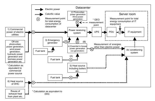
Fig. 2-10: GEC measurement points and handling of the use of Green electric power / exhaust heat
