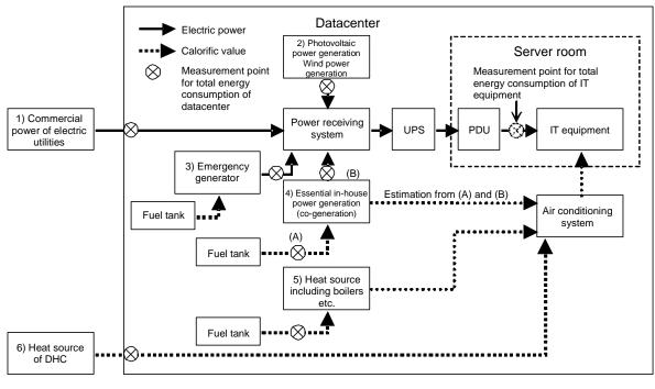
Fig. 2-7: Type of datacenter energy sources
