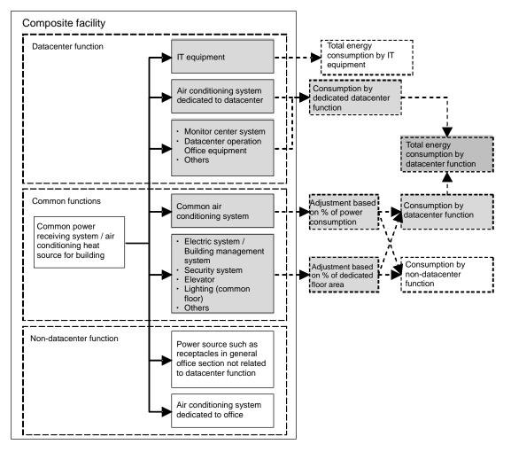
Fig. 2-9: Schematic image of a combined mixed-use type datacenter (non-Standalone), and how to determine the total energy consumption
