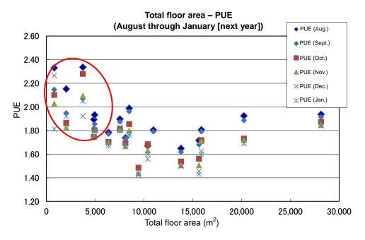
Fig. 3-4: Total floor size of datacenter building and the PUE
