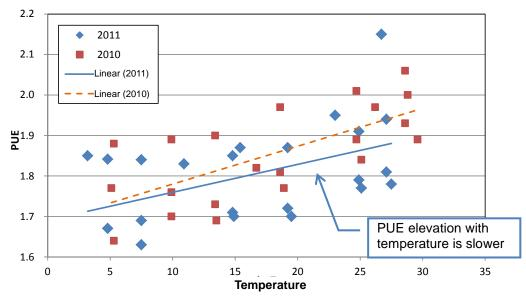
Fig. 3-6: Two years comparison of the PUE
