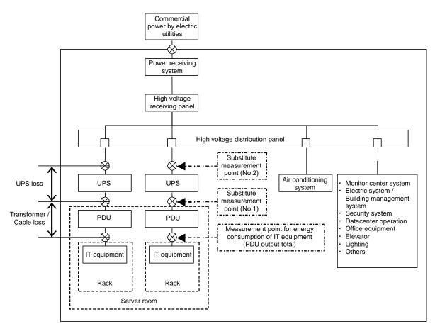
Fig. 2-8: Measurement points of IT equipment
