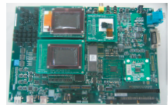
SH-Mobile evaluation board with TPM chip
