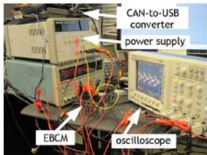
Figure 1. Example bench setup within our lab. The Electronic Brake Control Module (ECBM) is hooked up to a power supply, a CAN-to-USB converter, and an oscilloscope.
