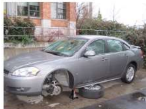
Figure 3. To test ECU behavior in a controlled environment, we immobilized the car on jack stands while mounting attacks.
