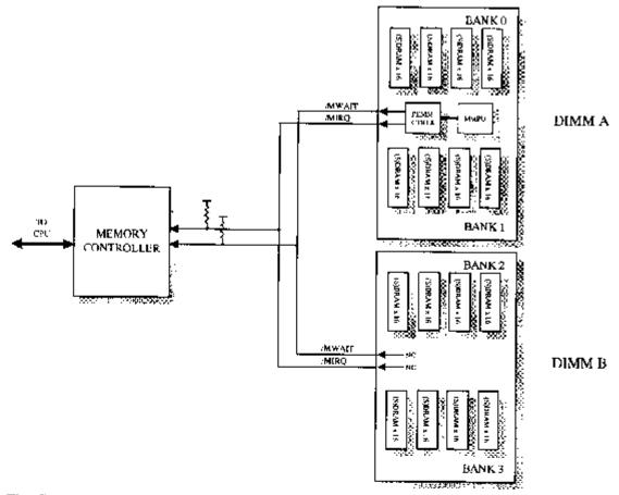
The figure above shows a typical block diagram for a 2-DIMM system using a PEMM. In this figure, DIMM A is a PEMM, and DIMM B is a standard memory module. As can be seen, the /MWAIT and /MIRQ signals shall be driven by the PEMM Controller(s) and wire ORed on the motherboard before being received by the Memory Controller.
