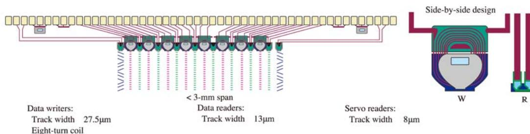
Ultrium I chip image schematic showing writers, readers, servo elements, and tracks. A 5-in. wafer contains 476 modules (238 heads). Each module is 22.5 mm × 0.75 mm (two per row). There are 16 interleaved write and read elements on a 166.5-μm pitch.
